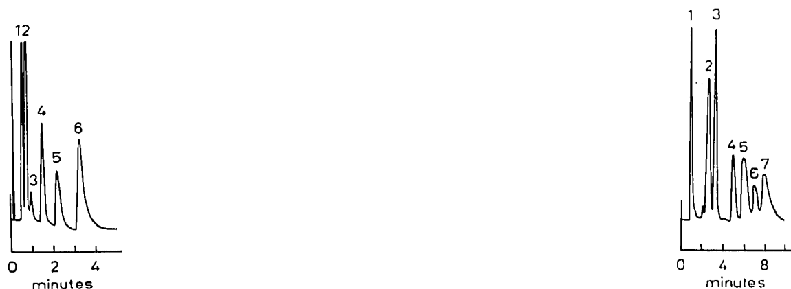
Fig. 8. Separation of tetracyclines. Column packing, SAS-Silica ( 6\ \mu\text{m} ); column dimensions, 125\ \text{mm} \times 5\ \text{mm} I.D.; eluent, 0.01 M \text{HClO}_4 in acetonitrile-water (14.5:85.5, v/v); pressure, 1000 p.s.i.; temperature, ambient; wavelength, 280 nm. 1 = 4-Epitetracycline; 2 = tetracycline; 3 = chlortetracycline; 4 = 4-epianhydrotetracycline; 5 = anhydrotetracycline. (Reproduced by permission of J. Jurand 48 .)
